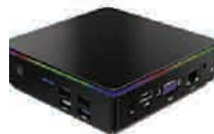
Gambar 4.5 Contoh Mini PC, Coffee Lake-U-based Bean Canyon Intel NUC8i5BEK2
